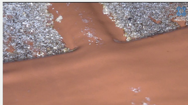
The surface of the vessel should be smooth and free from residue. The dent causes residue to get stuck.
