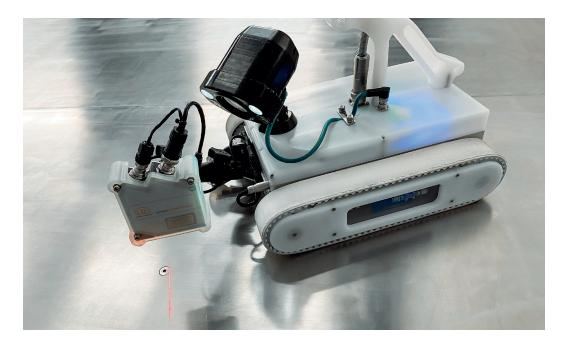
Accurately assess and size defects such as denting, scratches or pitting detected during visual inspection of assets, using innovative 2D scanning technology.
